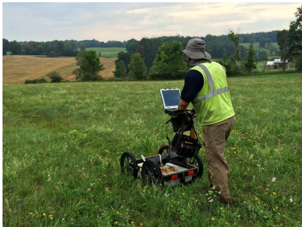
Collection of GPR Data
